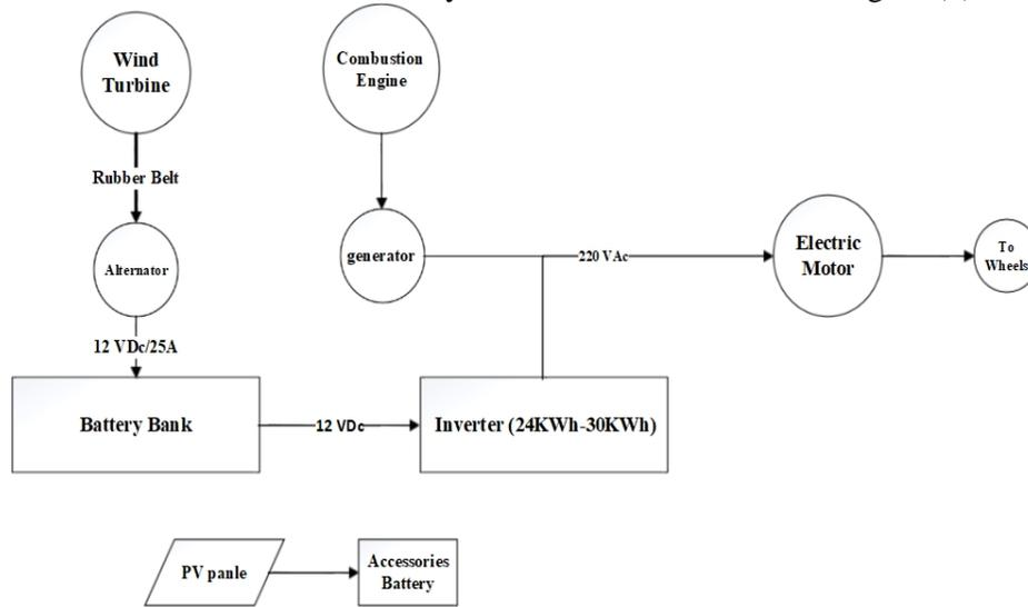
**Figure 5.**The studied model of hybrid vehicle.
