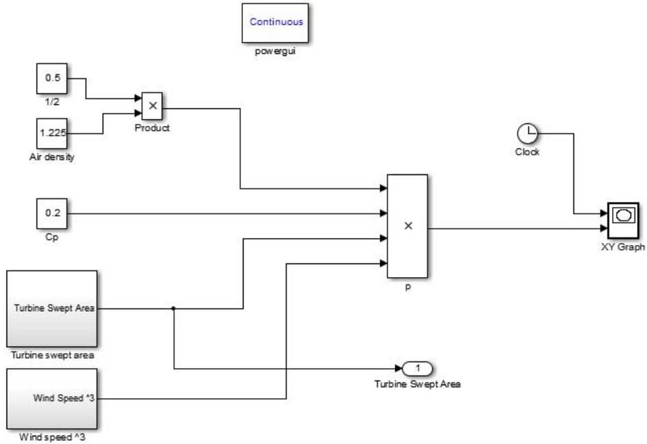
Figure 9. MATLAB Simulink model to calculate wind turbine output power.
