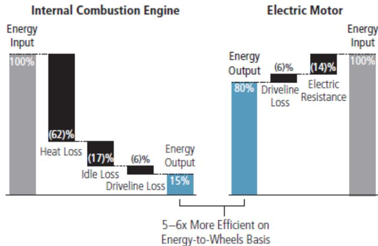
**Figure 1.** Electricity efficiency compared to combustion engines in powering cars.
