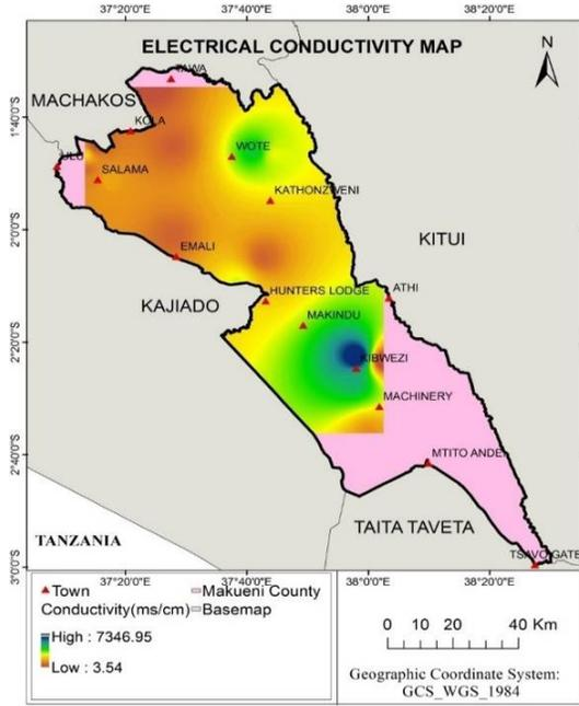
Figure 3 (a). The electrical conductivity map of the study area.
